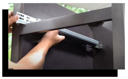
14. Once both slides have been secured to the drawer box, pull out both slides and place on the drawer box, make sure to fit the drawer box's back notches to the slides first. Pull the slides all the way up to the drawer clips until you hear a "click" sound confirming that the slides are secured to the clips. Repeat for the last 2 drawer boxes.
