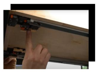
15. If you wish to remove the drawer box later, simply press the two white pieces on the drawer clips and the drawer box can be lifted off and removed from the slide rails.
